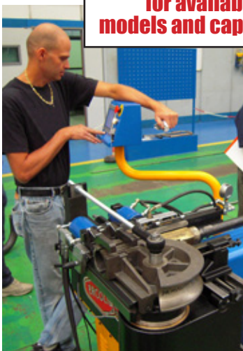
TM76 – Control offers easy access to manual and auto operating modes, system diagnostics and multiple languages.
