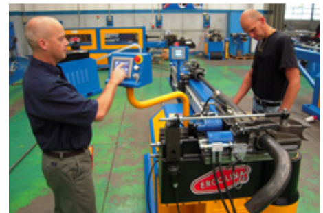
TM76 – Control offers easy access to manual and auto operating modes, system diagnostics and multiple languages.
